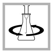
**6.** Put the end of the delivery tube fully into the solution. Swirl the flask. Turn the knob on the Digital Titrator to add titrant to the solution. Continue to swirl the flask. Add titrant until the color changes to colorless. Record the number of digits on the counter.
