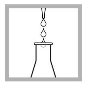
**3.** Use a pipet to add 25 mL of sample to a clean, 50-mL Erlenmeyer flask.
