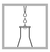
**3.** Use a pipet to add 25 mL of sample to a clean, 50-mL Erlenmeyer flask.
