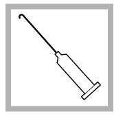
1. Insert a clean delivery tube into the digital titration cartridge. Attach the cartridge to the Digital Titrator.
