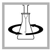
7. Put the end of the delivery tube fully into the solution. Swirl the flask. Turn the knob on the Digital Titrator to add titrant to the solution. Continue to swirl the flask. Add titrant until the color changes to colorless. Record the number of digits on the counter.
