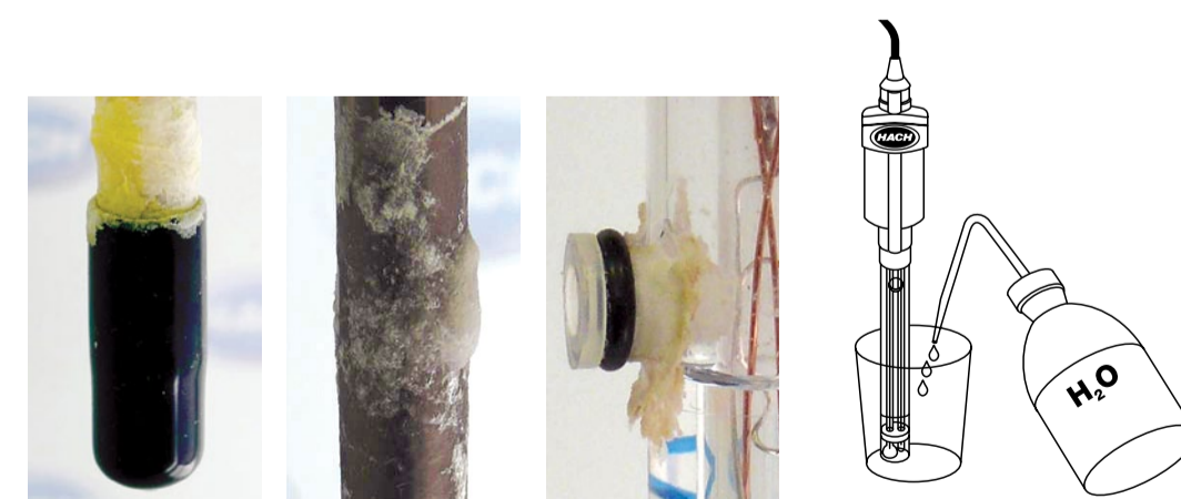
Innocuous crystallisation on storage cap, electrode shaft or refill opening
