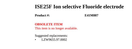
ISE electrode for measuring Fluoride concentrations from 0.01 - 20000 ppm. Temperature range 0 - 60 °C.
